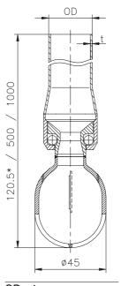
OD x t Welded on pipe 1" ISO: Ø25 x 1.2 Weld end\*
